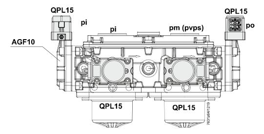
Example: Possibilities of fitting the QPL25 with nipple to the VGD20.xx3 Rp1/4"...1/8"
