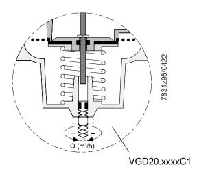
Q ( $m^3/h$ ) corresponds to approx. 5...100%. The adjustment can be made when the SKPx5 is activated.
